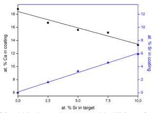
**Fig. 2** Incorporation of Sr ( $\blacktriangle$ ) in the coating measured by XPS as a function of the at. % of Sr in the target, and consequent decremental effect of the Ca ( $\blacksquare$ ) content in the coatings.
