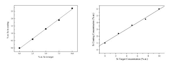
Fig. 3 Similar behaviors were found for *i*HA:Si and *i*HA:Se coatings obtained by laser ablation.
