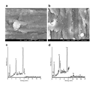
**Fig. 1** SEM micrographs and EDS analysis of two representative coatings deposited on titanium: pure HA (a,c) and *i*HA:Sr produced from an ablation target of 10% Sr (b,d).
