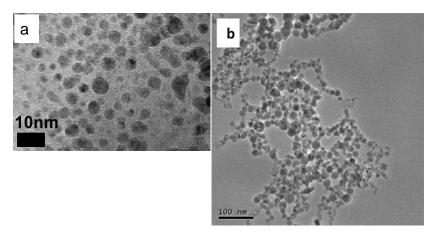
Fig. 3. TEM micrographs showing a) HA and b)  $TiO_2$  nanoparticles produced by laser ablation.
