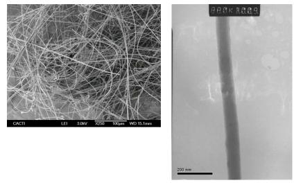
Fig. 4. SEM and TEM micrographs showing and overall view and a detail of the micro- and nanofibers of 45S5 Bioglass® produced by Laser spinnig.
