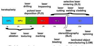
Fig 1. Laser assisted processes as a function of pulse duration.
