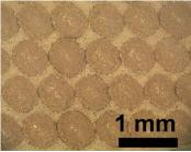
Fig. 2. Laser texturing of PEEK.
